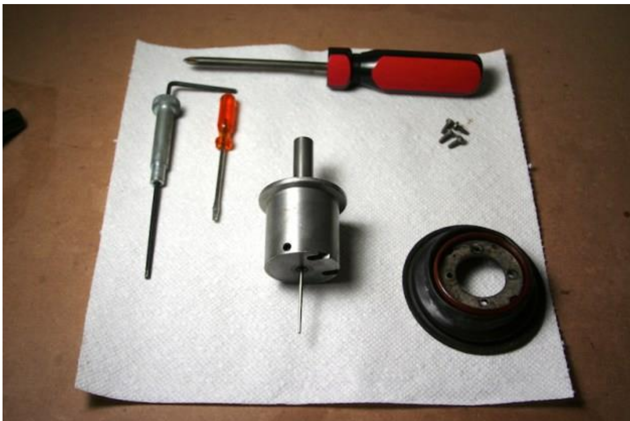
Tools, including a metering needle adjustment tool.
