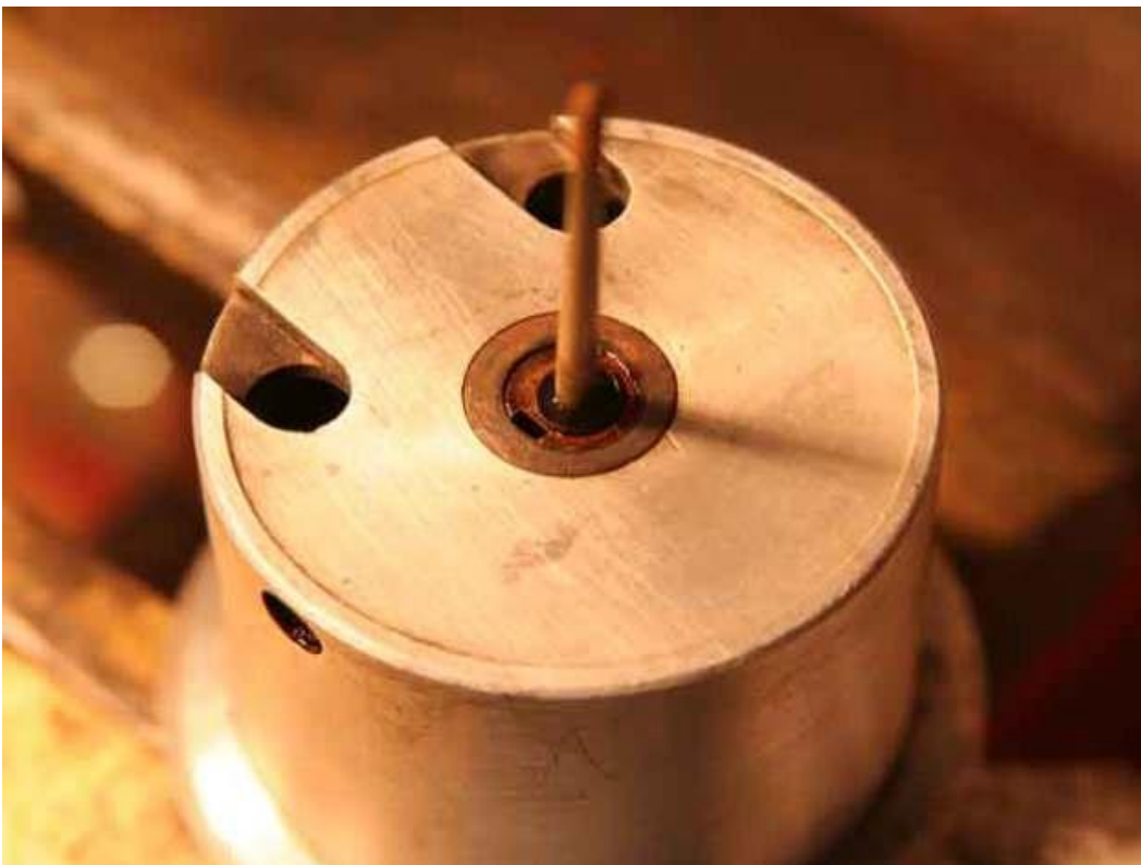
Closeup of the metering needle still in the piston.
