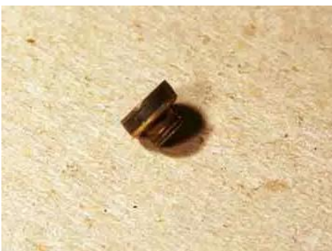
The needle adjustment screw. NOTE: the O-ring.
