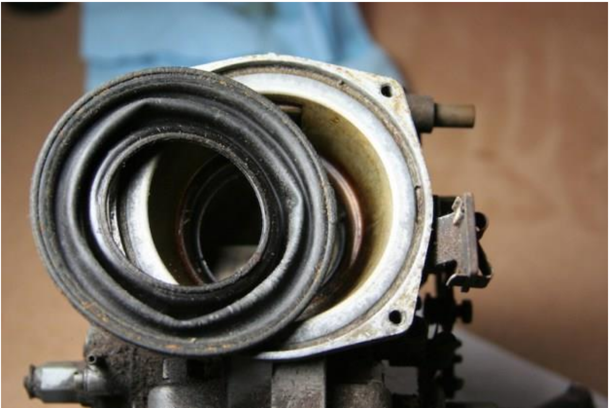
Alignment tab and groove on the carburetor bowl.
