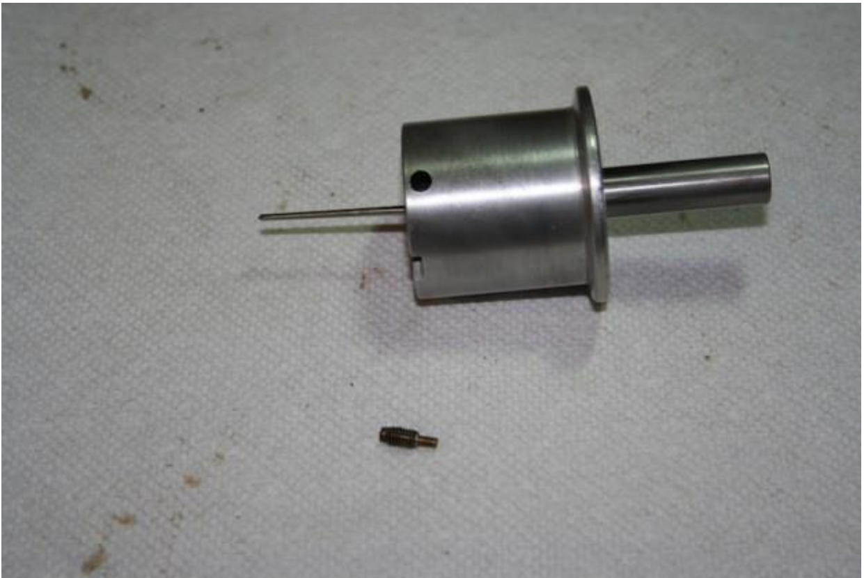
The retaining screw is tiny. It is found on the orifice shown above on the side of the piston.
