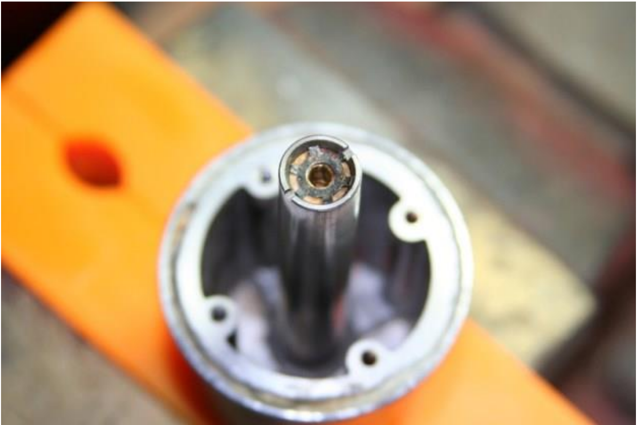
Closeup of the star washer with the metering needle adjustment screw below it.
