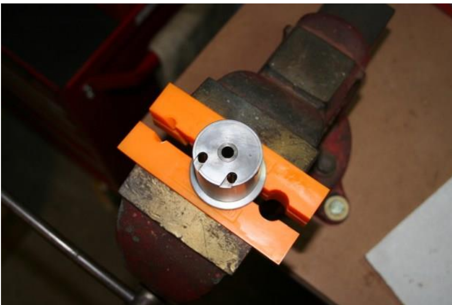
Brass housing for the metering needle
